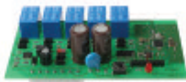
Wireless Energy Management Digital Thermostat Control Board: Snaps directly on to PTAC control board – no tools required.
