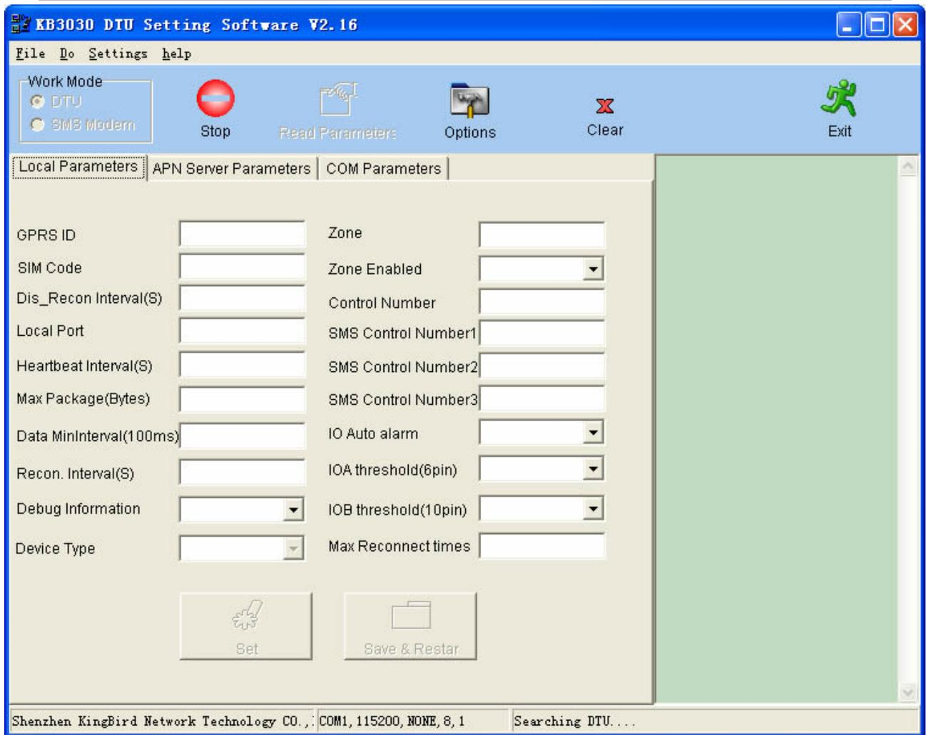
3. This software will automatically open corresponding serial search DTU, processing, please confirm whether the serial port which opened by software is the serial port connected with KB3060 DTU, if not, please click the “stop” button in toolbars in the menu options from the file, then change information in COM parameters settings window. (Note: configuration parameters are fixed by 115200bps)
