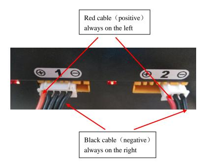
The above sketch is shown by a 4-cell and a 2-cell batteries connected in two ports. Also you can connect a 6-cell battery in one port, or 3 pcs 2-cell in different port, or 2pcs 3-cell batteries to different port. Shown by sketch below:
