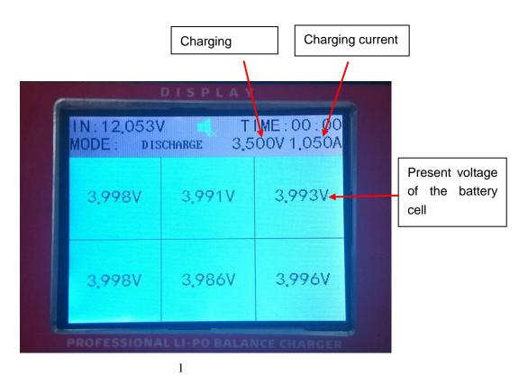
(2) Press the key SET, set the mode CHARGING or DISCHARGING. Press the key "+/▲"or"-/▼" to set voltage of discharging. Below sketch shows discharging setting interface: (discharging current is not settable, and charging voltage and current can set by yourself)
