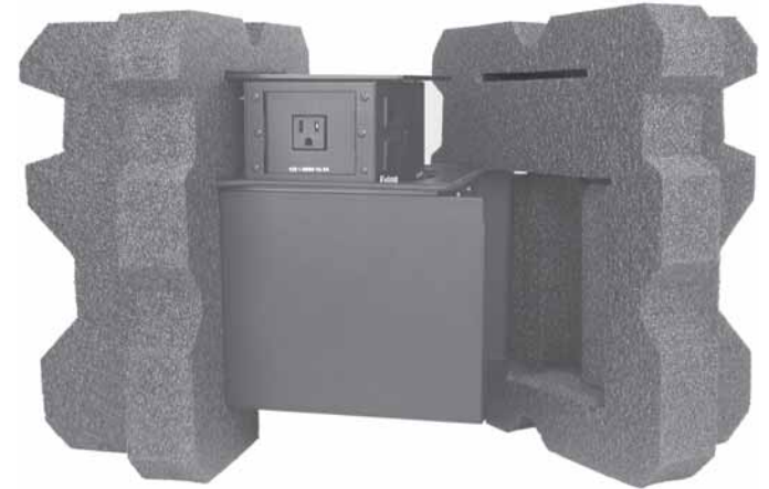
Figure B-5 — Installing the foam shell
