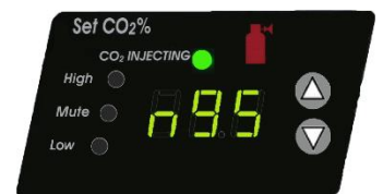
Figure 12: No Gas Supply
