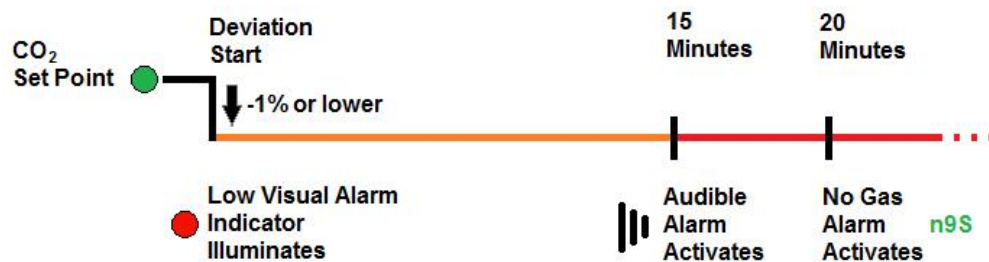
Figure 11: Gas Alarm Timeline
