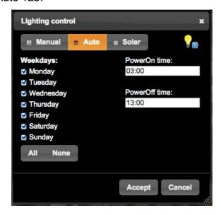
With Auto Lighting control the system will switch the courtesy lighting ON and OFF at the selected times on the selected days.
