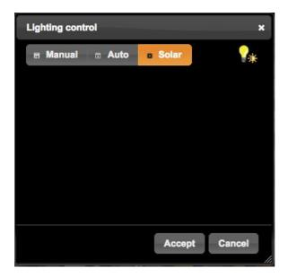
With Solar lighting selected the courtesy lighting will be operated by the solar control if installed.
