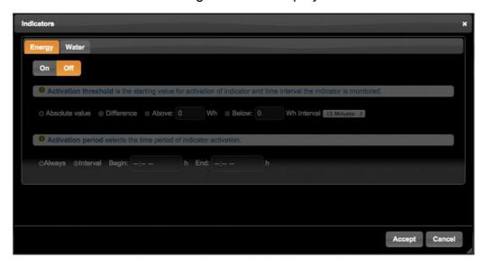
The window has Energy and Water tabs that allow control of monitoring for each supply. Click on either tab to configure the desired monitoring setting. Both tabs are identical in appearance except the Energy tab value is in Wh (watt hours) and the Water tab value is L (litres).
