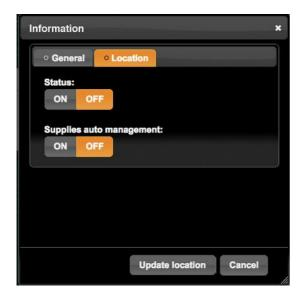
Set the Status to ON to inform the system that a CCRUM Locator module is installed in the vessel at the selected berth. Supplies auto management ON indicates that the utilities will be automatically activated when the CCRUM Locator is detected and off when not.
