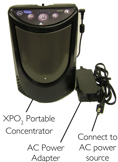
FIGURE 6.7 Powering the XPO 2
