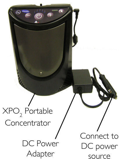
FIGURE 6.7 Powering the XPO 2
