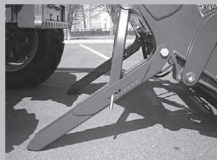
6- Parking props on the ground
