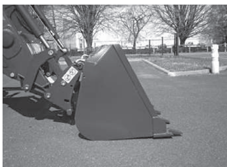
4- Tool flat on the ground
