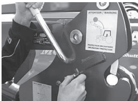
7- Unlock the loader
