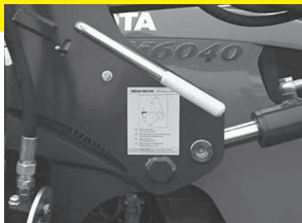
Right bearing box
