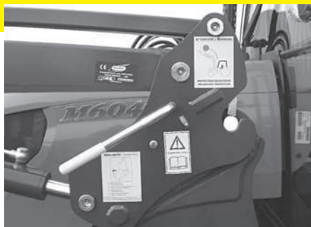
Left bearing box
