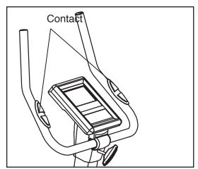
on the handgrip pulse sensor, remove the plastic. In addition, make sure that your hands are clean. To measure your heart rate, hold the handgrip pulse sensor with your palms resting against the metal contacts. Avoid moving your hands or gripping the contacts tightly.
