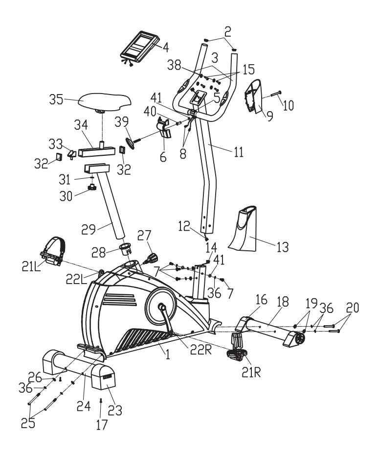
EXPLODED DRAWING—Model No. PFIVEX87112.0 part 2
