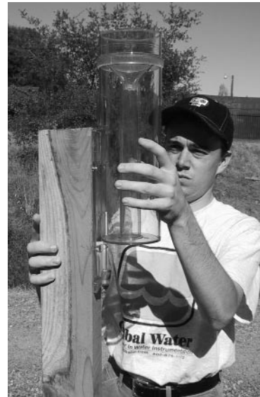
Slide the rain gauge into the mounting bracket.
