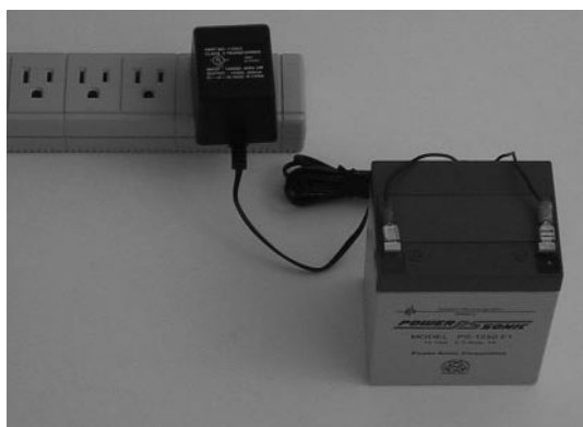
To recharge the battery, fasten the charger's disconnects onto the battery terminals and plug the charger into a wall socket.
