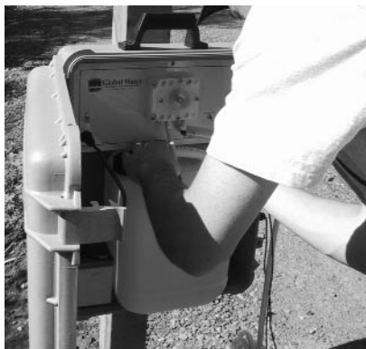
Place sample bottle into the carrying enclosure.
