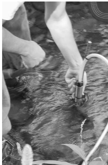
In a stream, the pickup strainer should be submerged under water.
