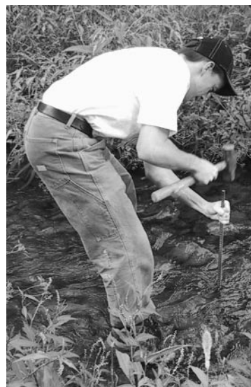
Securely insert a piece of mounting material into the center of the channel.
