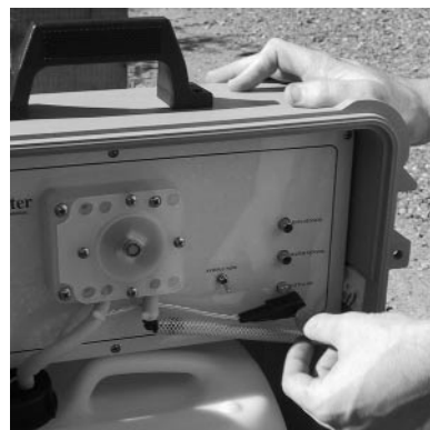
Plug the lead from bottle cap into "Bottle SW" socket.
