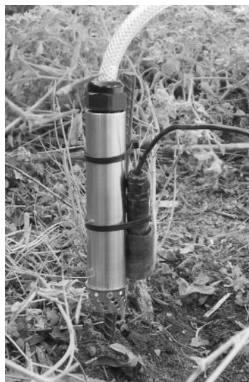
In a dry channel, the water sensor should be tied just above the debris strainer.
