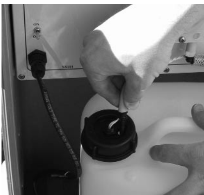
Insert end of peristaltic pump hose into the hole in bottle cap.
