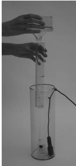
To trigger a sample when rainfall accumulates at 1.0 inch, insert the sensor in the outer cylinder at the depth as marked.
