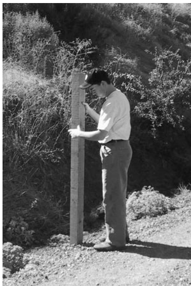
Install a 4" x 4" post that is located conveniently for daily readings.
