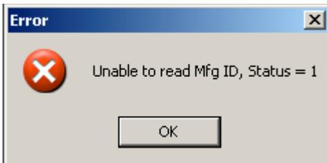
Press "Retrieve Locomotive Information..." a second time. Possibly the first "Retrieve" operation failed because the locomotive was executing an automatic reset to factory defaults, which can happen when you first install a new chip or upgrade the chip to new firmware.
