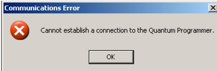
Make sure the USB cable is connected to your PC and to the Quantum Programmer. Make sure that another program which connects to the Quantum Programmer, such as QuantumCVManager, is not running.
