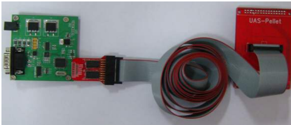
Figure 7.3 Connect UAS-Pellet Adapter cable to the User Board
