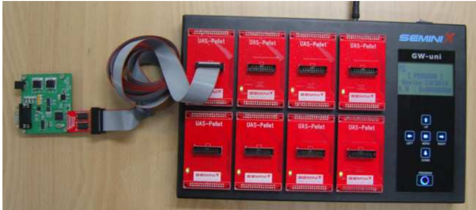
Connect GW-uni to User board via UAS-Pellet Adapter Cable
