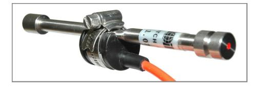
When the mounting blocks are welded in place the strain gauge is now positioned into the holes of the mounting blocks, ensure that the grooved end of the gauge lies inside the mounting block without the slot and the gauge is orientated so that the coil and clamp are not in contact with the structure.
