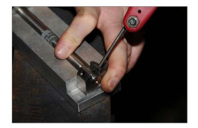
The steel surface is cleaned using a wire brush to remove all scale, rust, dirt and oil. The blocks are then removed from the spacing jig and pressed firmly against the steel surface using the setting bar as a handle. The edges of the mounting blocks are now welded.
