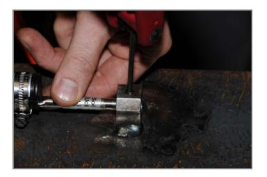
The cone point set screw should be tightened hard down into the V groove in one end of the gauge. Note: Do not rotate the gauge once the end has been clamped by the set screw.
