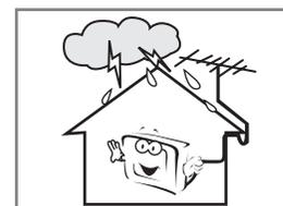
If an outside antenna is connected to the unit, ensure the external to internal cable entry is fully sealed
