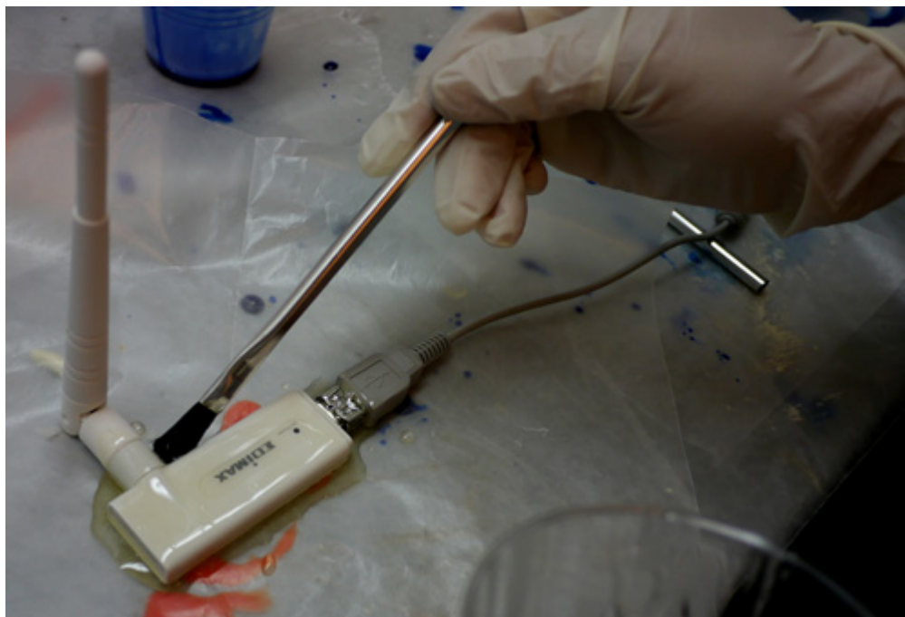
Figure 8: Coating connections in epoxy. Be sure to coat all joints and points of connection.
