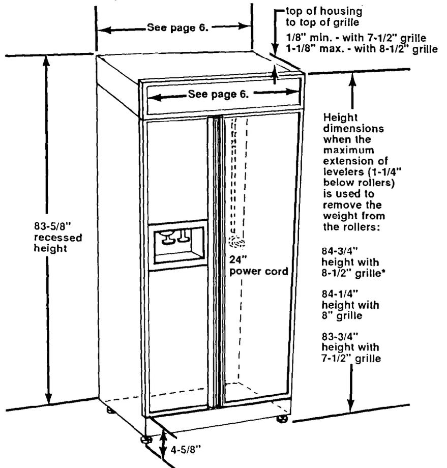
Height dimensions when the maximum extension of levelers (1-1/4" below rollers) is used to remove the weight from the rollers:
