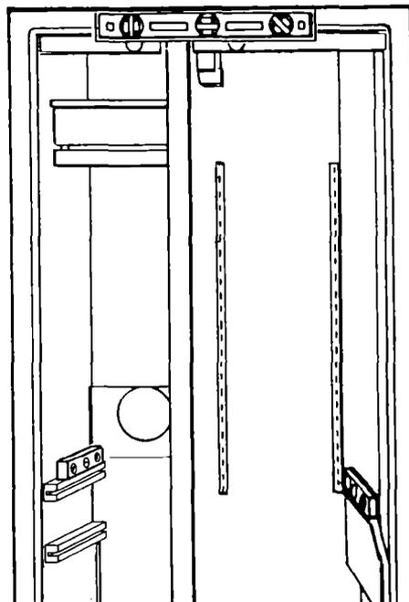
**Refrigerator must be level for proper operation. Important: All four leveling legs must contact the floor to support and stabilize the full weight of the refrigerator.**
