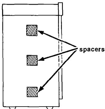
1. Attach three spacers from the miscellaneous parts bag to the top, middle and bottom of each side of the refrigerator. Spacers are required for ventilation.
