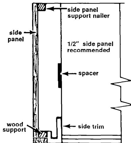
3. If less than 25" depth is available, side panel installation will need to be completed according to each site's restrictions.
