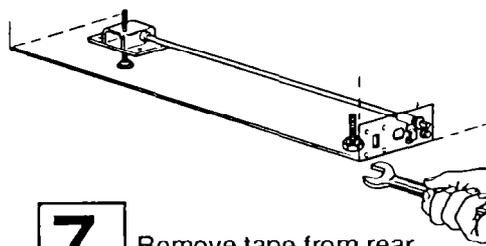
**7.** Remove tape from rear leveling rods. Turn the two leveling rods clockwise using a 5/16" socket and ratchet until the cabinet weight is supported by the rear legs. Use 1-3/8" open end wrench to lower the front leveling legs until the weight of the cabinet is supported by legs.
