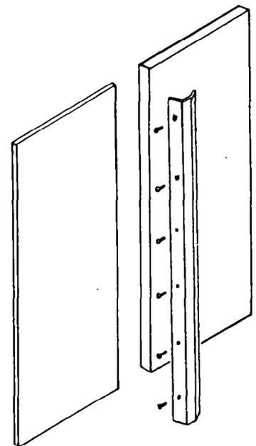
**10.** Remove all tape and door bracing from refrigerator door. Remove the six screws that attach the handle to the door frame. Slide the refrigerator door panel into door frame. If the panel is less than 1/4" thick, a filler panel will need to be installed between the door and decorative panel. If the decorative panel is more than 1/4" thick, it will have to be routed to have a 1/4" edge on all sides. See Custom panel and insert dimensions for exact sizes to cut custom panels.
