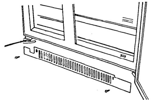
**15.** Open both doors. Use two screws to attach bottom grille to cabinet.
