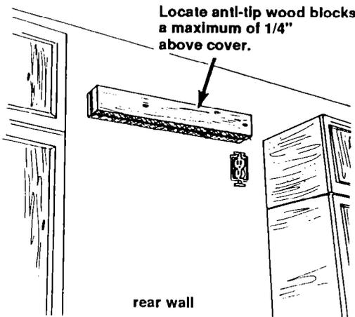
When a soffit is not available, locate wall studs in the refrigerator opening. Center one wood block and use wood screws to attach the wood block to the wall studs. Make sure screws engage wall studs a minimum of 1-1/2". Screw the second wood block to the front of the first block. The wood blocks must extend 2 inches beyond the ends of the cover.
