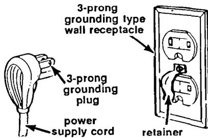
**5.** Move refrigerator close to final position. Remove cardboard or plywood from under refrigerator. Plug electrical cord into the grounded outlet. Use the screw from the parts package to install the plug retainer. Move the refrigerator evenly and straight into the opening. Check that the water line will not be kinked. Check that slack in the electrical cord hangs freely behind refrigerator or is placed on top of refrigerator next to cover.
