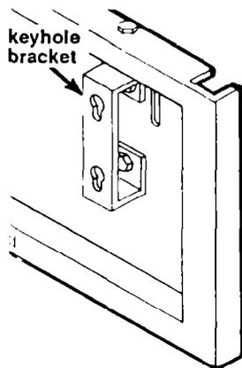
Check that the power switch is in the "ON" position. Attach top grille decorative panel assembly to the keyhole bracket on the frame and pull down to secure. If the top grille decorative panel does not fit evenly within frame, the keyhole bracket can be moved side to side by adjusting the bracket screws or the decorative panel bracket can be moved up or down by adjusting the decorator panel bracket nuts.
