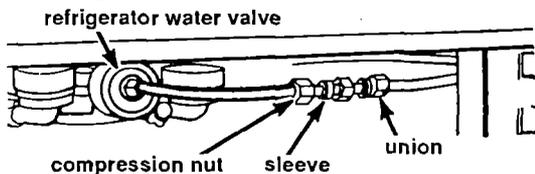
Connect tubing assembly fitting to refrigerator water valve. Do Not overtighten. (If necessary, water valve can be removed from underside of the cabinet to attach the fitting. You may have to remove the wiring channel to get to valve. Remove the screw between coils of water valve. Remove disconnected water valve and attach fitting. Replace the water valve.)
