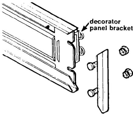
**11.** Remove two nuts from one end of the top panel frame. Remove end piece. Slide decorative panel into panel frame. Replace end piece using nuts.
