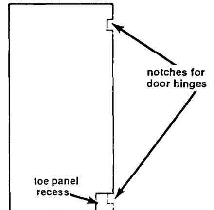
4. Height of side panels depends on your installation site. Side panels may need to be notched to clear door hinges. Side panels may be cut to match toe panel recess if desired.
