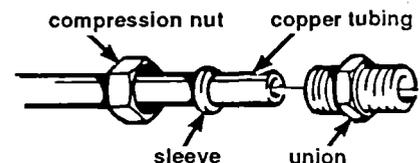
7. Slide compression nut and sleeve over water line.
