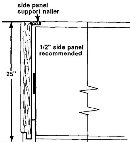
2. A side panel support nailer should be attached to the rear wall on each side of refrigerator
