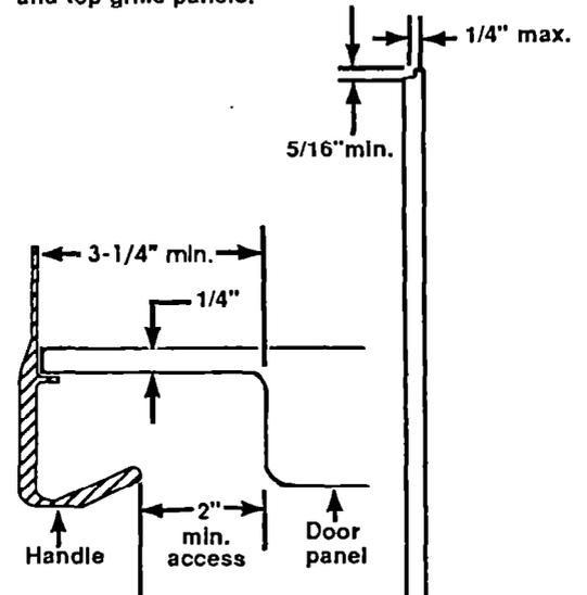
If custom door panels greater than 1/4" thick are used, it may be necessary to route the handle side of panel a minimum of 3-1/4 inches in from the panel edge to provide a 2" minimum access to the door handle. Either the full length of the panel or a selected area(s) can be routed. Check with your builder.
