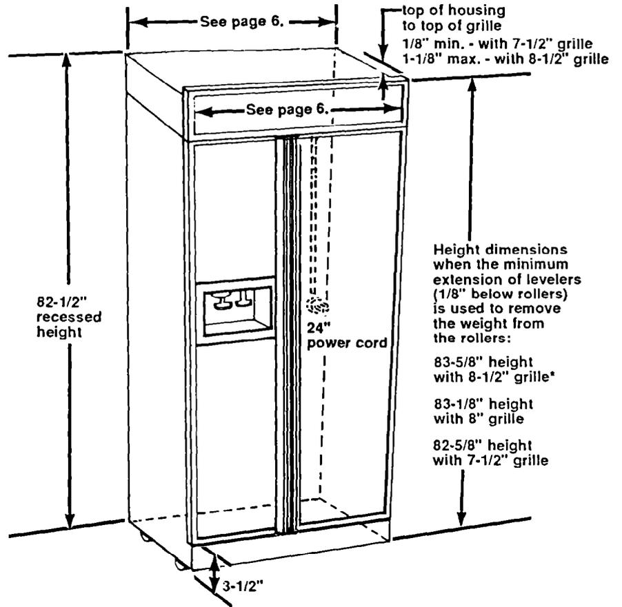
Height dimensions when the minimum extension of levelers (1/8" below rollers) is used to remove the weight from the rollers:
