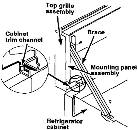
**12.** Attach the brace to the top right front corner of the refrigerator cabinet with one screw. Insert top grille flange into cabinet trim channel and align grille with top and side trim. Attach top grille mounting panel assembly to brace with one screw. Fasten grille in place with six screws.
