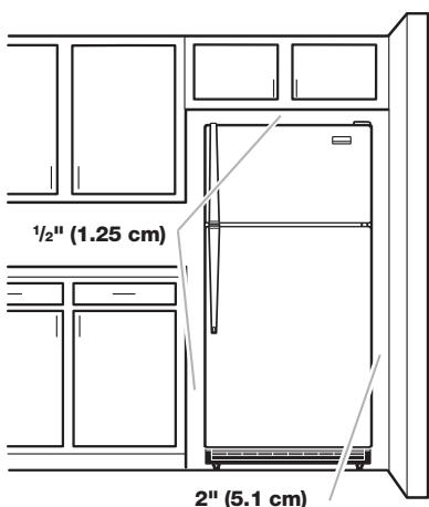
To ensure proper ventilation for your refrigerator, allow for a 1/2" (1.25 cm) space on each side and at the top. When installing your refrigerator next to a fixed wall, leave 2" (5.1 cm) minimum on the hinge side (some models require more) to allow for the door to swing open. If your refrigerator has an ice maker, allow extra space at the back for the water line connections.
