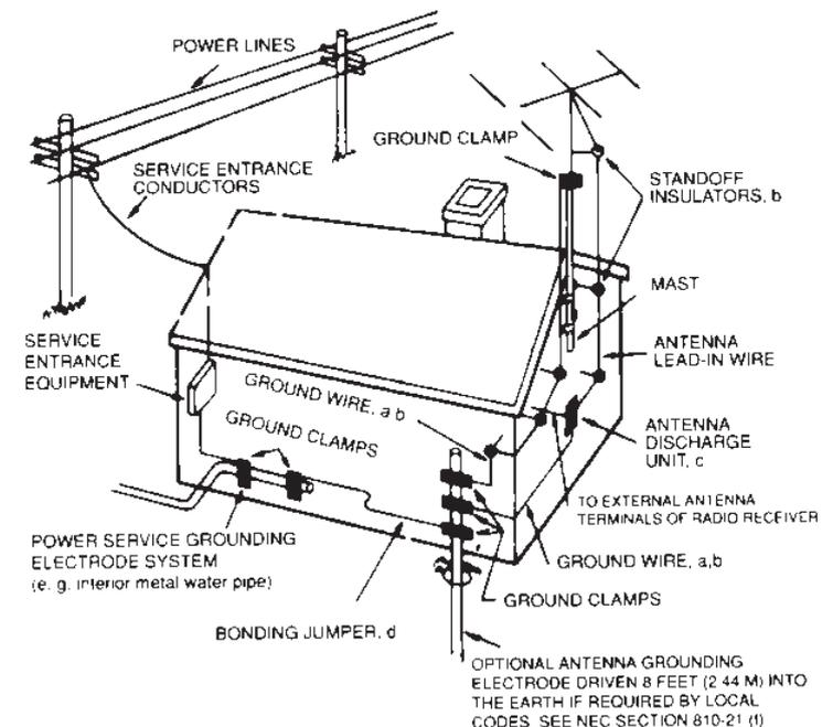
**NOTE TO CATV SYSTEM INSTALLER:** This reminder is provided to call the CATV system installer's attention to Article 820-22 of the National Electrical Code that provides guidelines for proper grounding and, in particular, specifies that the ground cable ground shall be connected to the grounding system of the building, as close to the point of cable entry as practical.
