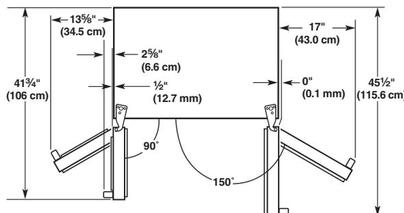
Location must permit doors to open to a minimum of 150°. Allow 13-1/4" (34 cm) minimum space between the side wall and the freezer side of the refrigerator. Allow 16-1/2" (42 cm) minimum space between the side wall and the refrigerator side.
