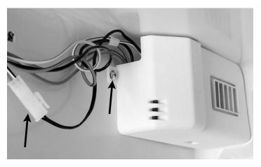
4. Remove the lead from the strain relief.
