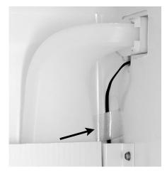
**Style 2 -** For models without ladders, the thermistor should be placed behind the air scoop assembly 7.8" (20 cm) down from the freezer compartment ceiling. Tape the thermistor lead to the freezer liner.
