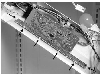
**4.** Disconnect the wire connectors and carefully remove the board from the control panel.
