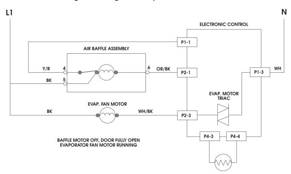
When the refrigerator thermistor reaches the cutout temperature, the control energizes the baffle motor to close the door.
