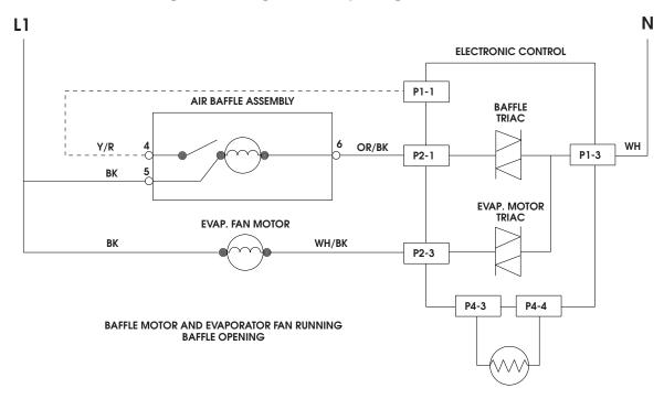
When the baffle door is fully open, the switch closes sending 120vac out pin 4 (Y/R wire) on the baffle door assembly to pin P1-1 on the control. When the control senses 120vac at P1-1, the motor stops with the door fully open.
