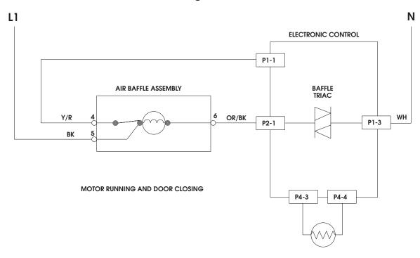
When the baffle is fully closed, the switch opens interrupting power to P1-1. This signals the control to stop the baffle motor with the door fully closed.
