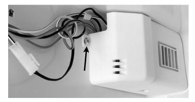
**4.** Locate the air chute in the top of the freezer compartment.
