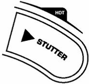
**Play/Stutter:** Starts the music from either the first set cue point or the last point of pause. By starting from the last pause point while the unit is paused a new cue point is set. Pressing this button while the unit is in play restarts the unit from the last cue point, creating a “stutter” effect.
