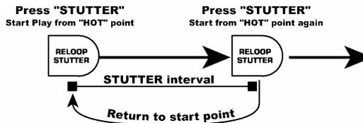
**NOTE:** The CD Player will always remember a new set "Hot" points until you actually set a new "LOOP IN" point or put in a new CD. The new point will be accessible until you remove the CD from the unit.
