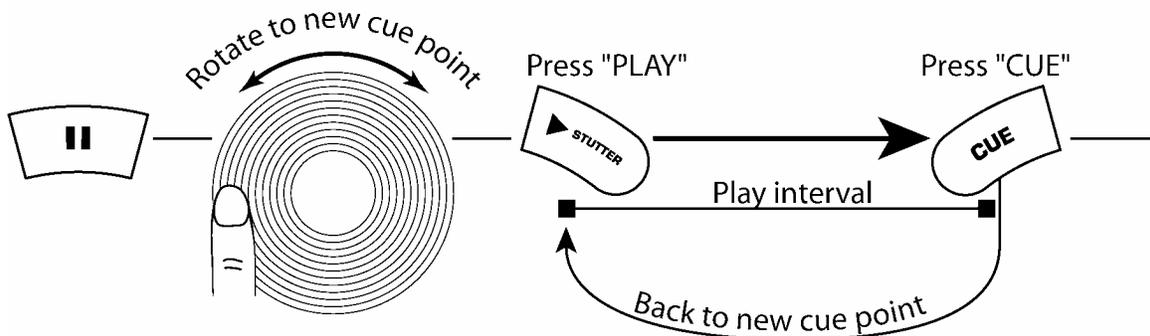
When the jog wheel is turned while paused, a new cue point can be located. By pressing "PLAY" while paused that point will be set. By pressing "PLAY" again (STUTTER) the point can be checked as desirable.
