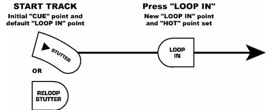
**NOTE: The CD Player will always remember a new set point as the "LOOP IN" or "HOT START" point until you actually set a new "LOOP IN" point or put in a new CD. The new point will be accessible until you remove the CD from the unit. If**
