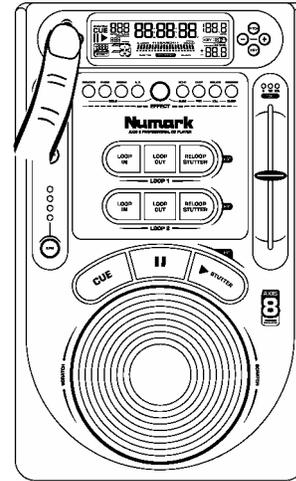
Switch off the power **after** the disc holder has been closed with the "OPEN/CLOSE" button
