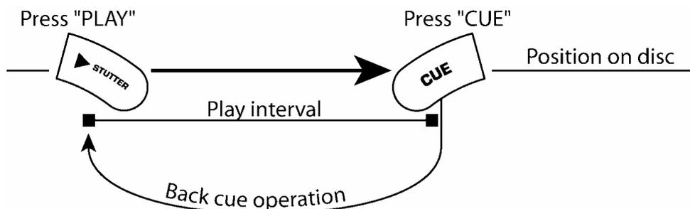
Pressing the "PLAY" button starts the disc. Pressing the "CUE" button will reset the disc to the last place where the disc was started. This is called the cue point. By alternately pressing the "PLAY" button and the "CUE" button, the disc may be returned and played from the cue point any number of times. This function is called back cue.
