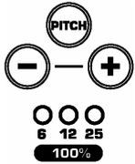
**Pitch Range:** activates the pitch slider and adjusts the amount of control the pitch slider has on the overall speed of music. On depression of will toggle the slider on and off. Range adjustments of 6, 12, 25, and 100% can be achieved by holding down and then pressing to cycle through the range options. *This setting will be remembered at power down.*
