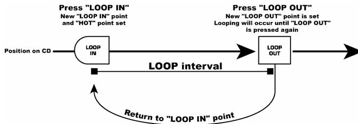
**Note: The "LOOP OUT" point will be erased if "LOOP IN" is pressed or a new "CUE" point is set after the "LOOP OUT" point. This is important because without this point "RELOOP" will not be possible.**
