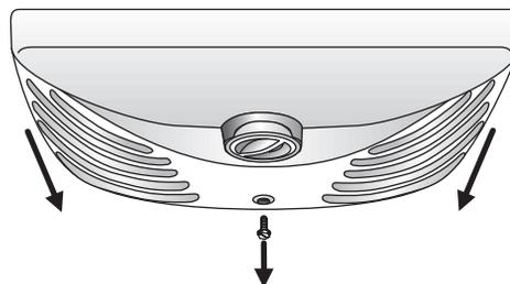
4. Replace burned-out bulb(s) with an appliance light bulb no greater than 40 watts.
