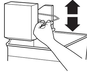
2. Install the interior water filter cartridge. The interior water filter mounting bracket is located on the top right side of the refrigerator compartment.
