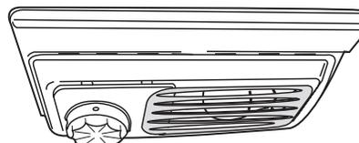
3. Replace burned-out bulb with appliance bulb no greater than 40 watts.
