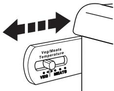
**IMPORTANT:** If food starts to freeze, move the control to the left (less cold). Remember to wait 24 hours between adjustments. Doing so gives the temperature of the food time to change.
