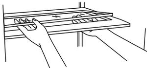
3. Replace back of meat drawer cover frame into supports or slides on side walls of the refrigerator and lower or slide the front of the cover frame into place.
