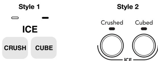
For crushed ice, cubes are crushed before they are dispensed. This may cause a slight delay when dispensing crushed ice. Noise from the ice crusher is normal, and pieces of ice may vary in size. When changing from crushed to cubed, a few ounces of crushed ice will be dispensed along with the first cubes.
