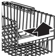
3. Replace the basket or bin by positioning it on the side wall guide rails. Lift the basket or bin front slightly while pushing it past the guide rail stops and slide basket or bin in the rest of the way.
