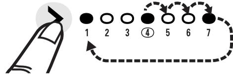
**NOTE:** With each press of the arrow, you will hear a beep as the light moves to the next setting. The indicator light moves to a setting of “7” and then returns to the setting of “1.”
