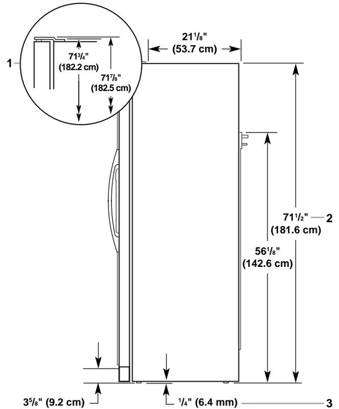
1. Dimensions shown from floor with rollers set at minimum height
