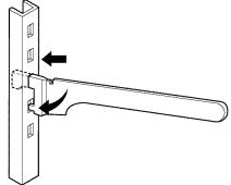
▲ CAUTION: Make sure that shelves are level from one side to the other. Failure to do so may result in the shelf falling or spilling food.
