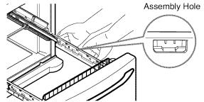
• With the drawer pulled out to full extension, insert the lower basket (4) in the rail assembly.
