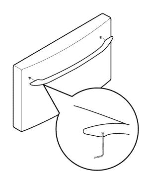
NOTE: It is "always" recommend that the doors be removed when it is necessary to move the refrigerator through a narrow opening. If it is necessary to remove the handles follow the directions below.
