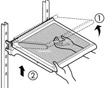
• To reinstall a shelf—Tilt the front of the shelf up and guide the shelf hooks into the slots at a desired height. Then lower the front of the shelf so that the hooks drop into the slots.
