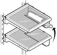
Bottle holder can be removed by pulling it straight out and installed by placing it at the end of the shelf you want and pushing it inward.
