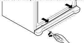
2. Turn the leveling leg clockwise to raise that side of the refrigerator or counterclockwise to lower it. It may take several turns of the leveling leg to adjust the tilt of the refrigerator.
