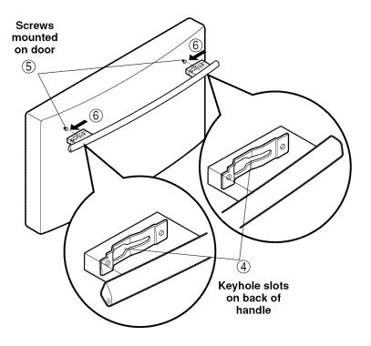
**NOTE:** It is "always" recommend that the doors be removed when it is necessary to move the refrigerator through a narrow opening. If it is necessary to remove the handles follow the directions below.
