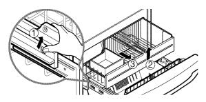
To install, reposition the gear part of rear left and right side of the drawer after pulling out both rails as much as possible, and gently push down both left and right side while checking the hook on the front part.
