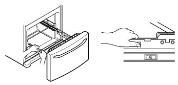
• Remove the screws(2) of the rail on both sides.
