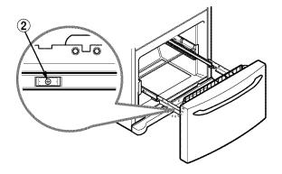
• With both hands, hold both sides of the door and pull it up to separate it from the rails.
