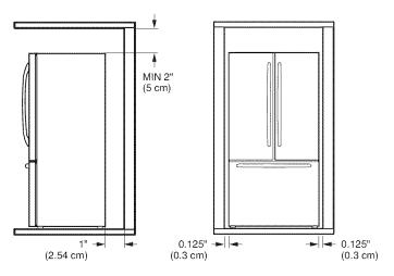
• Too small a distance from adjacent items may result in lowered freezing capability and increased electricity consumption charges. Allow at least 24 in. (61 cm) in front of the refrigerator to open the doors.
