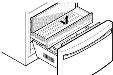
2. To replace, slightly tilt up the front of the drawer, insert the drawer into the frame, and push it back into place.
