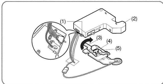
1. Open the door. Remove the top hinge cover screw (1). Lift up the cover (2).
