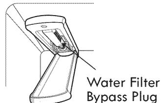
**CAUTION:** DO NOT operate refrigerator without water filter or water filter plug installed.
