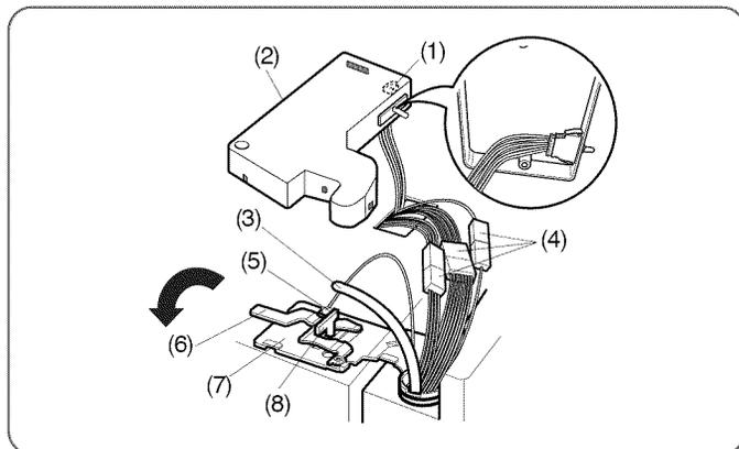
1. Open the door. Remove the top hinge cover screw (1). Lift up the cover (2).
