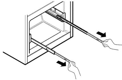
Grasp the drawer on each side and hook drawer supports ① into rail tabs ② located on both sides.
