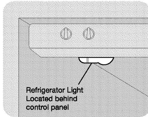
Refrigerator Light Located behind control panel
