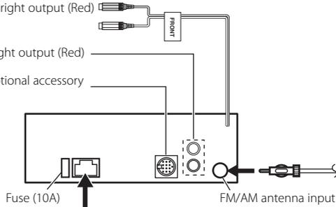
If no connections are made, do not let the wire come out from the tab.
