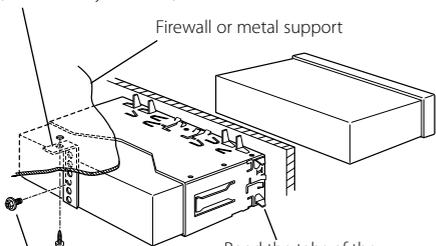
Bend the tabs of the mounting sleeve with a screwdriver or similar utensil and attach it in place.
