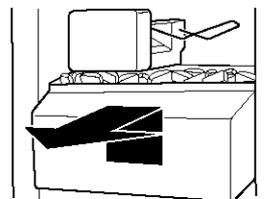
4. Replace the bin by pushing it in all the way or the dispenser will not work. Push the wire shutoff arm down to the ON position to restart ice production. Make sure the door is closed tightly.
