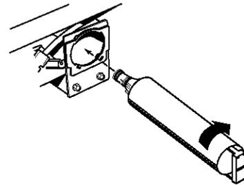
2. Take the new cartridge out of its packaging and remove protective cover from o-rings.
