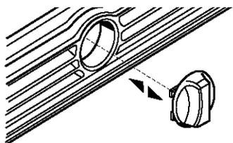
3. Rotate the cartridge cap to a horizontal position. The cartridge cap might not be even with the base grille.
