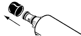
4. Slide the cartridge cap onto the new cartridge. See illustration in Step 2.
