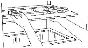
3. Replace back of meat drawer cover frame into supports or slides on side walls of the refrigerator and lower or slide the front of the cover frame into place.
