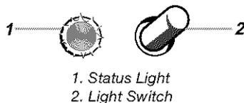
After changing the water filter cartridge, reset the water filter status light by pressing the light switch 5 times within 10 seconds. The status light will change from red to green when the system is reset.
