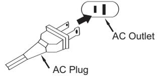
**NOTE:** The AC plug supplied with the unit is polarized to help minimize the possibility of electric shock. If the AC plug does not fit into a nonpolarized AC outlet, do not file or cut the wide blade. It is the user's responsibility to have an electrician replace the obsolete outlet.
