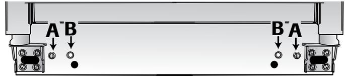
4. Turn both rear adjustment screws (B) clockwise to raise and counterclockwise to lower the rear of the refrigerator.
