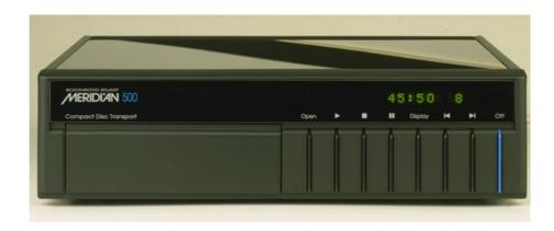
The 500 Compact Disc Transport incorporates a precision engineered CD turntable and drawer system, which provides all the advantages of drawer loading with the superior disc clamping normally associated with top loading players. It provides a precision digital output which is re-clocked and uses a very high power 75 ohms amplifier for superlow jitter.
