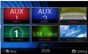
**[AUX1]**-Press the button to display the AUX1 mode.
