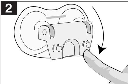
Pull the suction cup lever down and it will stick to the wall.
