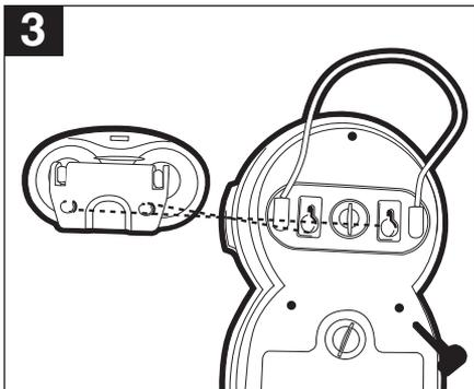
Connect the main unit to the Wall Adapter by inserting the holes on the base unit into the hooks on the Wall Adapter.
