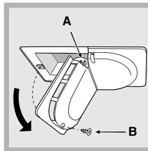
Access the light bulb (A) by unscrewing the fixing screw (B) which is located at the back of the lampcover, as shown (see diagram). Replace it with a similar light bulb, the power of which should not exceed 15W.
