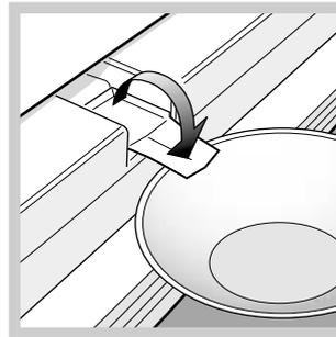
5. Certain appliances are fitted with the DRAIN SYSTEM to lead the water outside: insert the scraper into the slot provided at the bottom and let the water flow into a container (see diagram).
