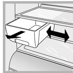
**MULTI-USE bin:** to store food (such as cold meats) for a long time and also prevent odours from lingering in the refrigerator. It can be removed for use and it may be shifted sideways to optimise space (see *diagram*).
