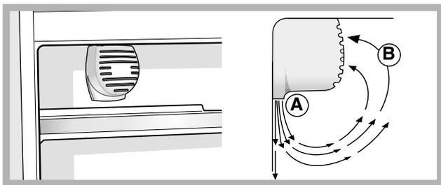
The A.I.R. System maintains a constant fridge temperature to keep food fresher for longer and will quickly restore the temperature to the correct level, even if the door is opened frequently: the blown air (A) is cooled when it comes into contact with the cold wall,
