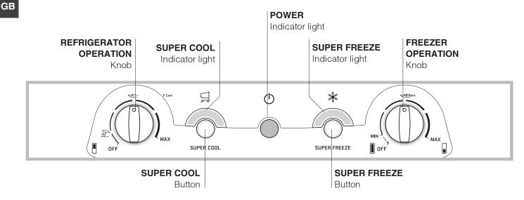
REFRIGERATOR OPERATION Knob to regulate the temperature of the refrigerator compartment.
