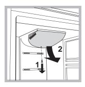
socket. Follow the instructions below. Access the light bulb by removing the cover as indicated in the diagram. Replace it with a similar light bulb within the power range indicated on the cover (15 W).
