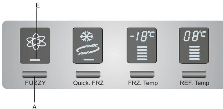
In the Intelligent operating mode, the temperature inside the appliance is adjusted automatically according to variations of the ambient temperature. Press key A once, upon which indicator E lights up and Intelligent mode is entered. Press key A once again, upon which indicator E goes off and Intelligent mode is cancelled.
