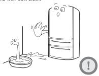
The refrigerator should be placed in a well-ventilated place not far from a drink water source. A space of at least 20cm and 10cm must be kept above and around the refrigerator.
