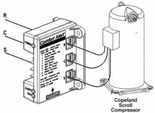
Comfort Alert™ is self-contained with no required external sensors and is designed to install directly into the electrical box of any residential condensing unit that has a Copeland Scroll™ compressor inside.
