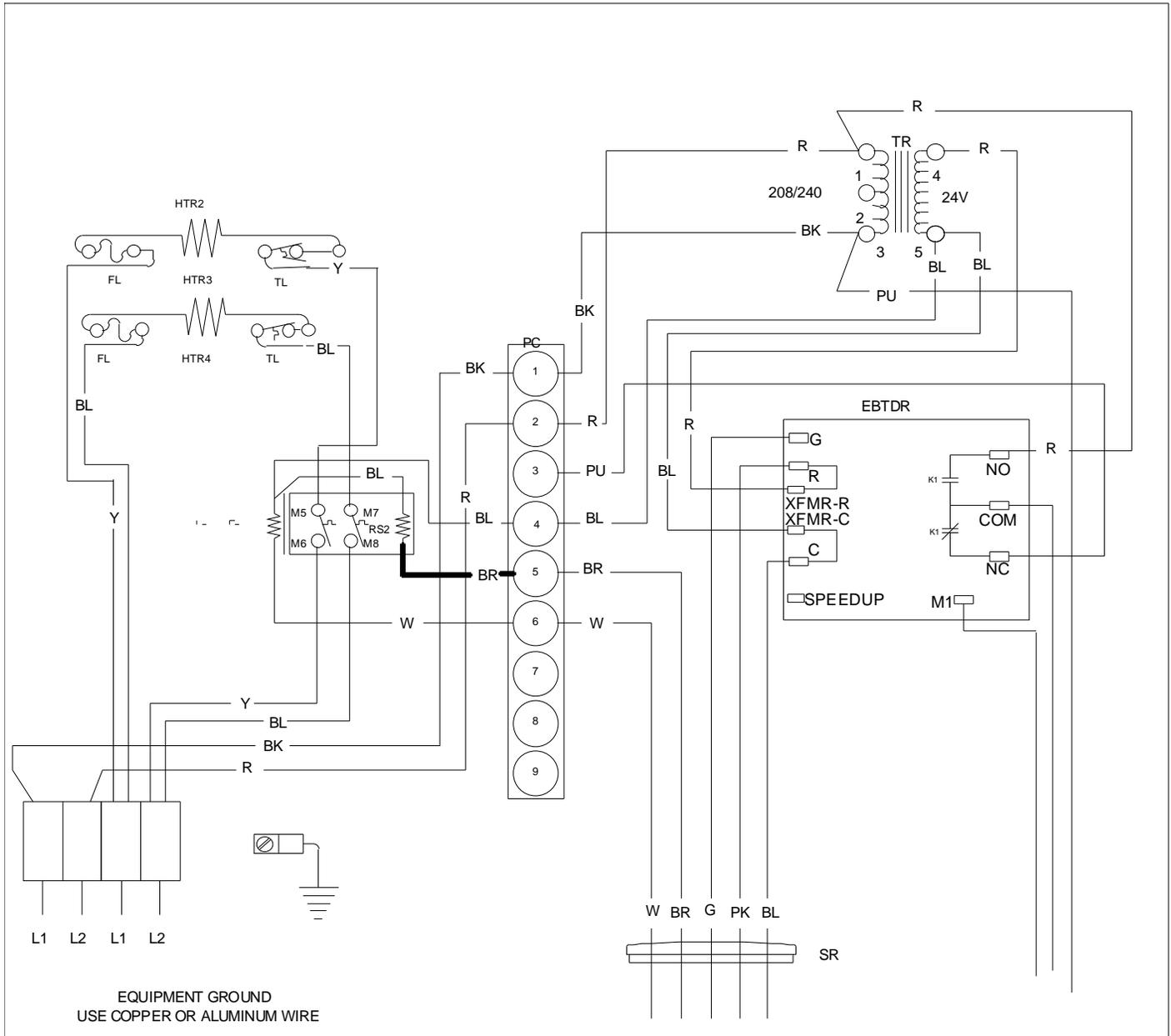
Typical Wiring Schematic MBR Blower with Electric Heat.
