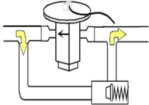
Most expansion valves used in current Amana® Brand Heat Pump products use an internally checked expansion valve. This type of expansion valve does not require an external check valve as shown above. However, the principle of operation is the same.
