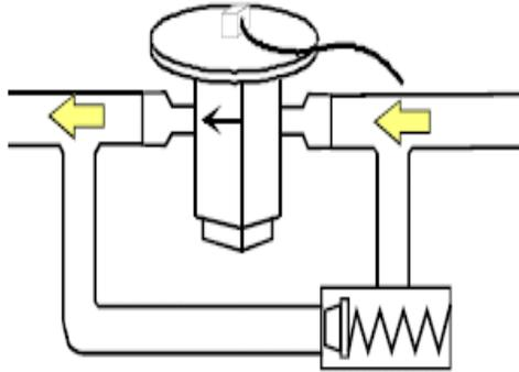
**EXPANSION VALVE/CHECK VALVE ASSEMBLY
