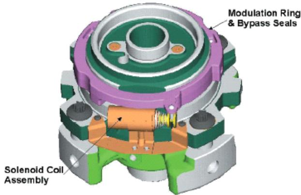
The ZPS/ZRS two-step modulated scroll uses a single step of unloading to go from full capacity to approximately 67% capacity. A single speed, high efficiency motor continues to run while the scroll modulates between the two capacity step
