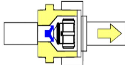
In the heating mode, the orifice moves back off its seat, allowing refrigerant to flow unmetered around the outside of the orifice.
