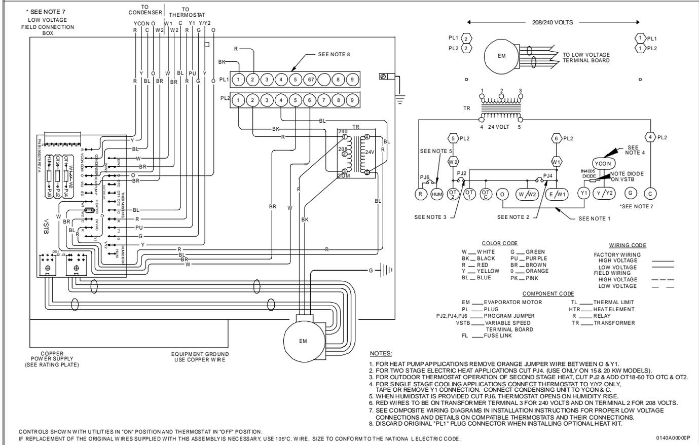
Typical Wiring Schematic AEPF with Electric Heat.
