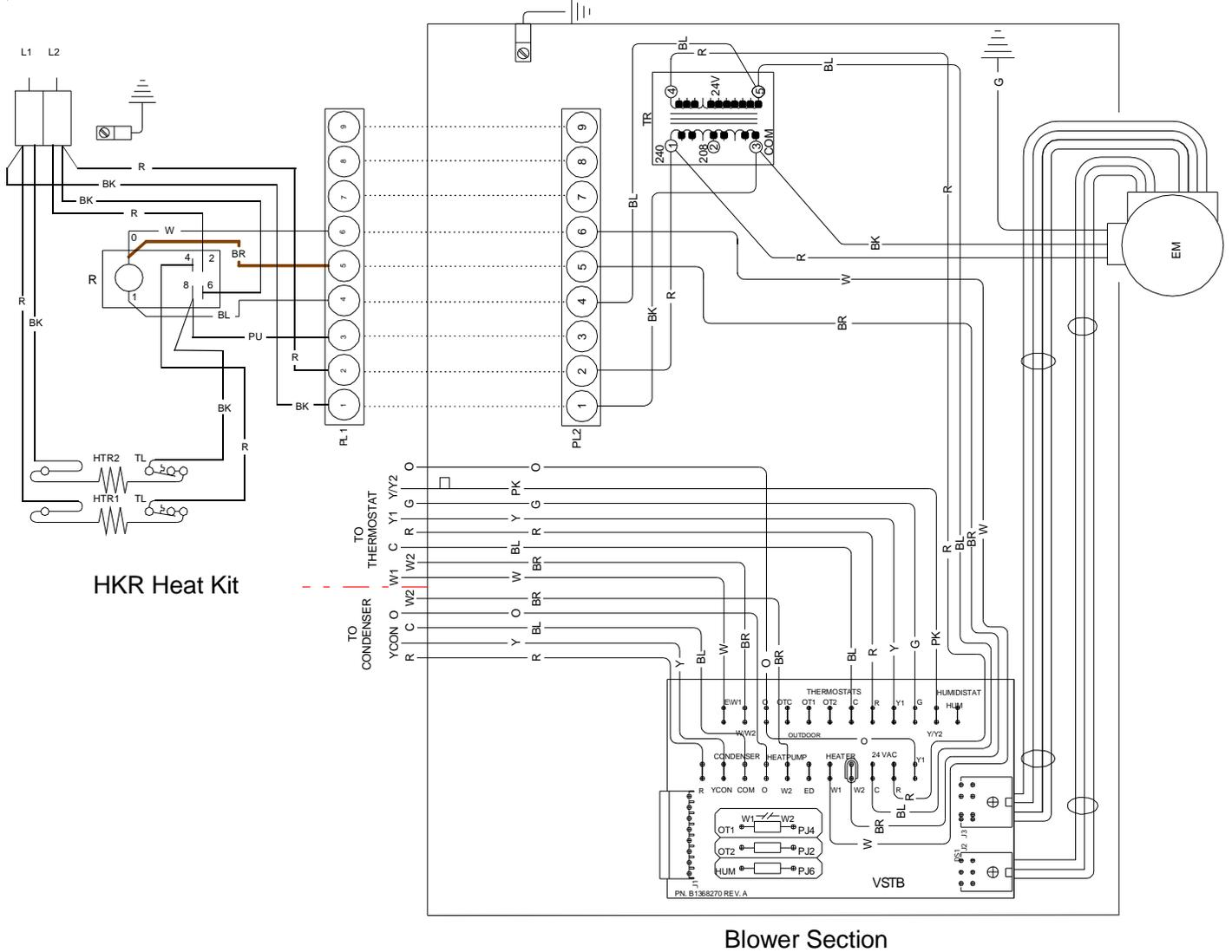
Typical Wiring Schematic MBE Blower with Electric Heat.
