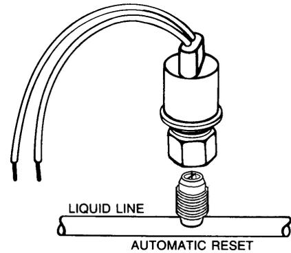
If it cuts-out at 610 PSIG  $\pm$  10 PSIG, it is operating normally (See causes for high head pressure in Service Problem Analysis Guide). If it cuts out below this pressure range, replace the control.
