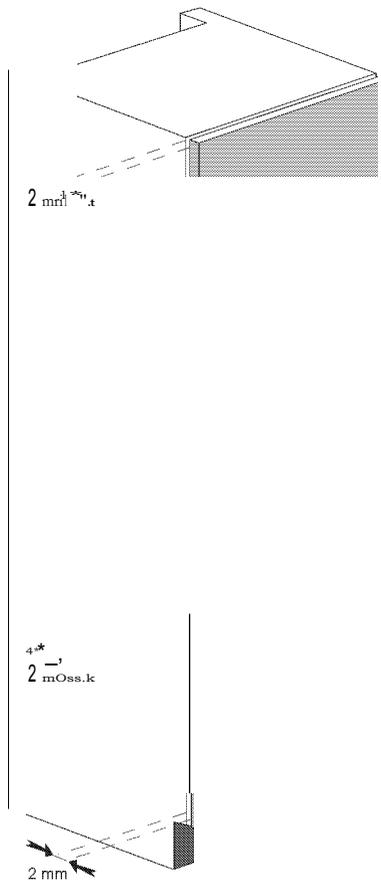
Ensure 2 mm gaps are obtained, adjust if necessary.
