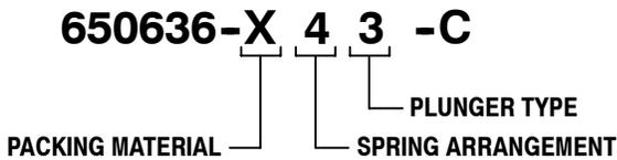
**PACKING MATERIAL** (PACKINGS ARE UPPER AND LOWER UNLESS NOTED)
