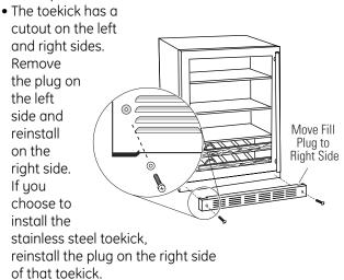
• Install original screws and spacers or screws and spacers supplied with the stainless steel toekick. Install screws through the spacer standoff, toekick and into the base as shown.
