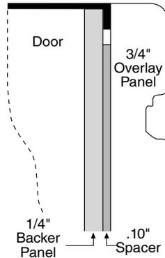
Center each panel over the other. Assemble the panels with glue and screws. Screws must be countersunk into the backer panel.
