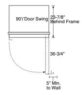
Allow 25" minimum clearance for a full 130° door swing. Allow 15" for pan removal. for a 90° door swing, allow 5" minimum clearance for professional models. If the 90° doorstop position is used, pan access is maintained but pan removal is restricted.
