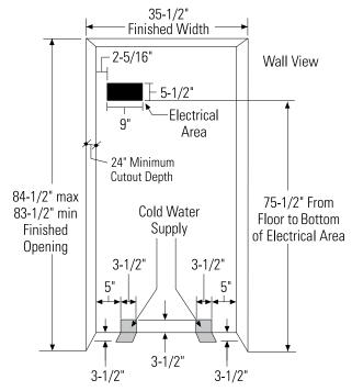
The water and electrical supply must be located as shown. The finished cutout width must be 35-1/2".
