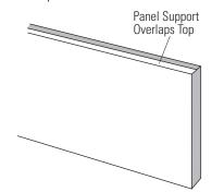
Back View Grille Panel Support • Install four of the six larger undercut screws so that the top of the screws are 1/16" from the surface of
