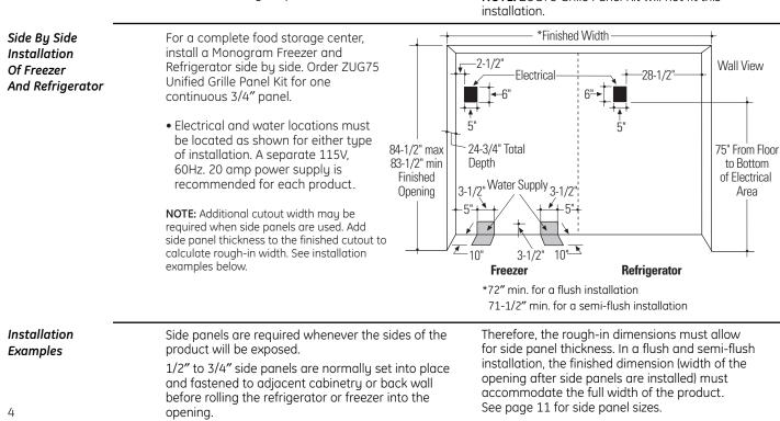
**Clearances for Multiple Single Door Installations** In a side-by-side installation of a left and right door swing product, no clearance between the units is required. If you are installing 3/4" thick custom panels, order ZUG75 Unified Grille Panel Kit for one continuous grille panel.
