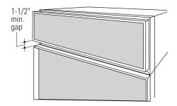
**IMPORTANT:** Maintain 1-1/2" min. gap between top of door and bottom of grille panel.
