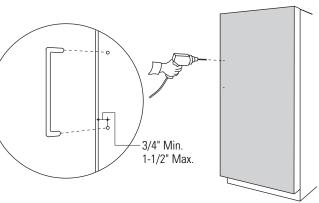
Step 3 Assemble panel, extrusion and handle
