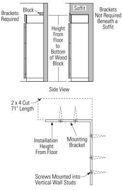
**IMPORTANT NOTE:** When the products are installed under a soffit or if there is not enough height for this method of security, use Step 4 as an alternative. **The refrigerator and freezer must be secured to prevent tipping.**
