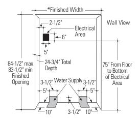
\*36" Min. for a flush installation 35-1/2" Min. for a semi-flush installation
