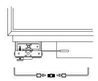
**NOTE:** Make sure excess tubing length does not interfere with toekick installation.
