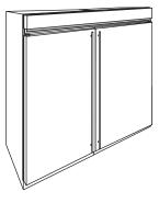
Side by side installation with 3/4" custom panels and unified custom grille panel. Trim Kits ZUG75, ZKTR36LH, ZKTR36RH.
