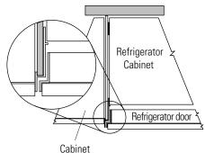
**1/4" Side panels –** Insert end of side panel into case trim. Fasten with stick-on hook and loop strips.
