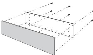
• Secure the grille panel support to the back side of the 3/4'' thick custom panel with #6 screws. Be sure the lip of the support is over the top of the wood panel.
