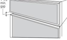
**IMPORTANT:** Maintain 1-1/2" min. gap between top of doors and bottom of panel frame.
