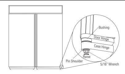
Check door alignment. The top of the door should be parallel with the grille panel. If the door appears to be too high or too low on the handle side, adjustments can be made.
