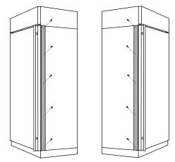
Install new side case trim with notches towards the bottom. Install with original screws.
