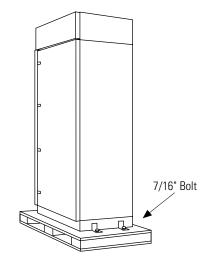
• Lift the refrigerator off the skid with an appliance dolly. Handle from the sides.
