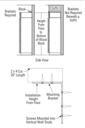
**IMPORTANT NOTE:** When the refrigerator is installed under a soffit or if there is not enough height for this method of security, brackets cannot be used. Proceed to step 5 to level the refrigerator and then to step 6 to secure refrigerator to cabinets. The refrigerator must be secured to prevent tipping.
