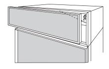
E. Mount the assembled panel by dropping into slots on the case trim.
