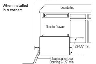
Allow 2-1/2" min. clearance between Double-Drawer and adjacent cabinet, wall or other appliances. Allow 23-1/8" min. clearance from the front for drawer opening.
