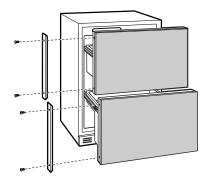
• Place the brushed decorative covers over the side trim to hide the screw heads. Ensure side trim is aligned top to bottom and front to back. Snap into place.
