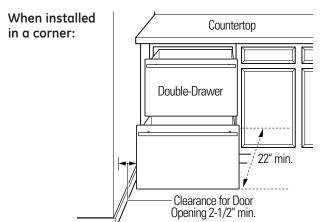
Allow 2-1/2" min. clearance between Double-Drawer and adjacent cabinet, wall or other appliances. Allow 22" min. clearance from the front for drawer opening.
