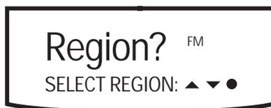
The CLASSIK Movie Di must be set for the correct radio frequency range for your country. Use the ▲ / ▼ keys on the handset to select your region (either Europe, USA or Japan) then press 'enter' on the handset. If you are unsure of the correct setting contact your local Linn retailer.
