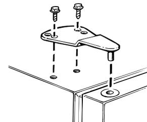
Installing the hinge on the left.
