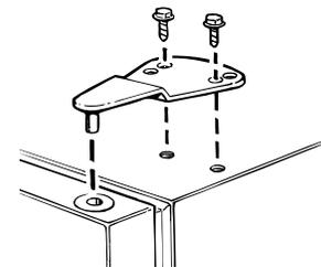
Installing the hinge on the right.
