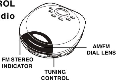
**NOTE:** If you tune into an FM stereo station, the FM STEREO indicator will be turned on.
