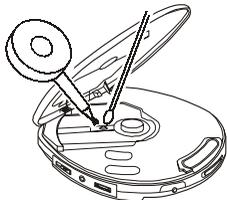
Use a cotton swab very slightly dampened with alcohol to clean the lens.
