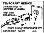
**TEMPORARY CONNECTION** may be made to a properly grounded two-prong **wall outlet** by use of a **UL-listed** adapter (**Fig.** 2), available at most local hardware stores.
